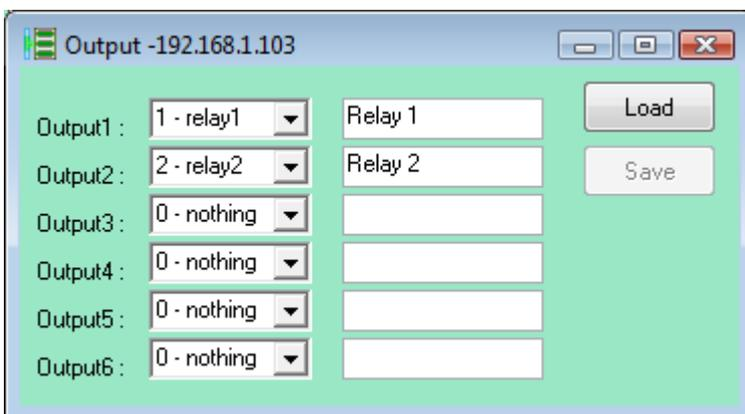
The screenshot shows a window titled "Output -192.168.1.103". It contains six rows of output settings. Each row has a dropdown menu, a text field, and a button. The first two rows are pre-filled: Output1 with "1 - relay1" and "Relay 1", and Output2 with "2 - relay2" and "Relay 2". The remaining four rows (Output3 to Output6) have "0 - nothing" in the dropdown and empty text fields. The Load and Save buttons are positioned to the right of the first two rows.
