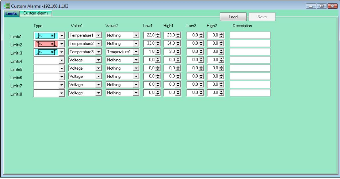
Limits are used to monitor values like limits on measurement. Use for setting thermostat, that enter into user alarms.
