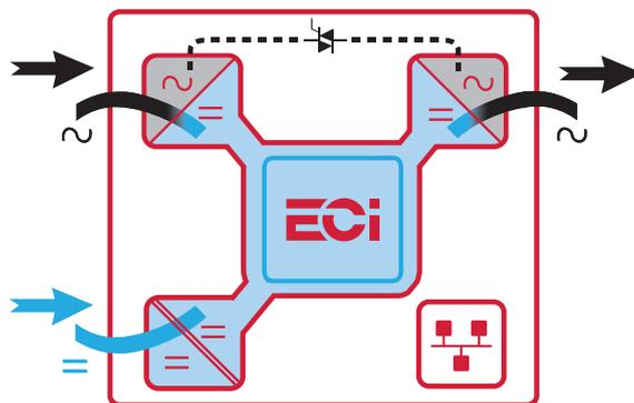
The ECI technology **eliminates all single points of failure** with full scalability; up to 32 modules in parallel and high efficiency of up to **96% in AC to AC conversion**, and above **93.7% in DC/AC conversion**, hence reducing operating costs. We can build the systems up to **2.7 MVA**.
