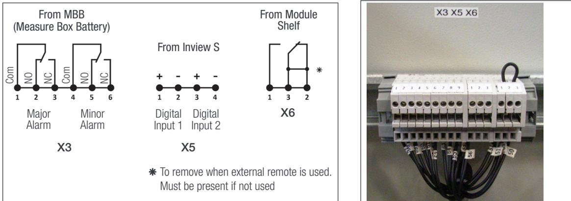
When an alarm occurs, the X3 relay contacts are de-energized and switch.
