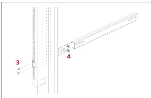
Assemble the sliders and adjust the length to suit the mounting depth.
