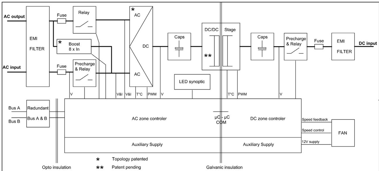
The module is built around the following sub-converters
